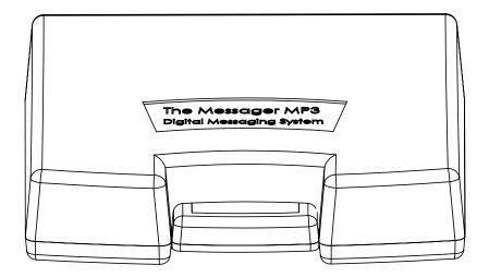
MESSAGE MATE SLOT - The slot on the front of the Messager MP3 accepts a proprietary flash memory cartridge which stores all of the MP3 files.
